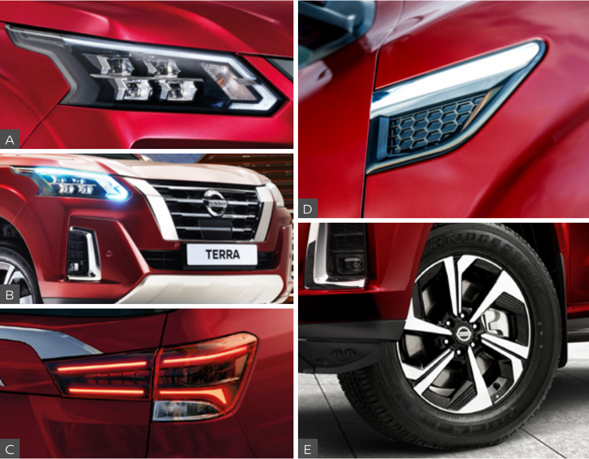
A Quad LED Projector headlamps with signature LED DRLs
